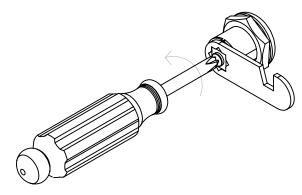
3. Keeping the sheet on the flat surface, rotate the padlock as shown in Fig. 2, so that the notch is inverted (See Fig. 1 and Fig. 2 to see before and after).
